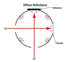
This procedure would result in a distorted absolute sample spectrum. Since the sample of interest and the standard reference have different absorption and scattering properties, exchanging them alters the reflectivity of the integrating sphere over the samples' surface areas. Due to the average reflectivity of the integrating sphere being different for the two measurements, they are not perfectly compatible.
